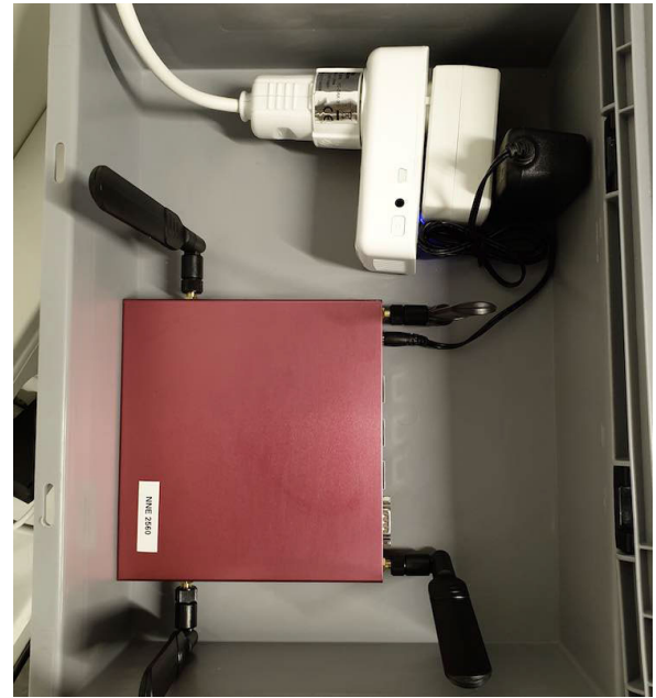
FIGURE 1. Measurement node. The red box encloses the single board computer. The box also includes a smart power socket that can be rebooted via SMS.
