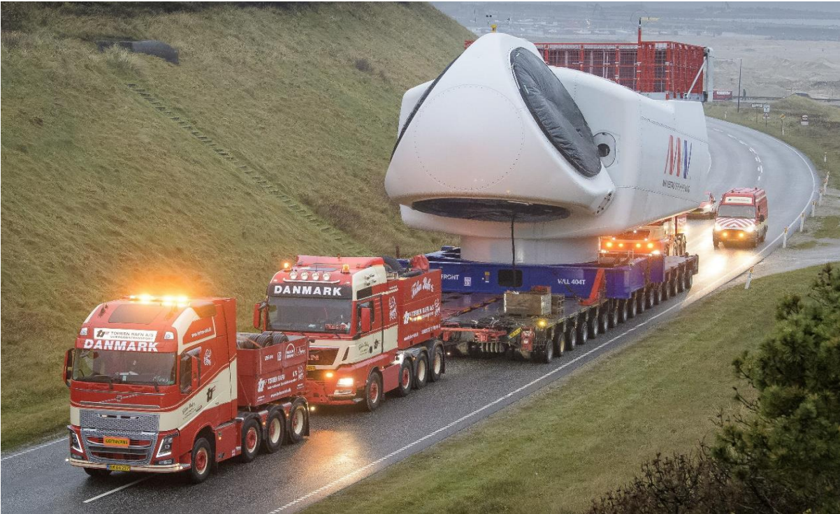
Figure 3.29: Onshore transportation of nacelle
