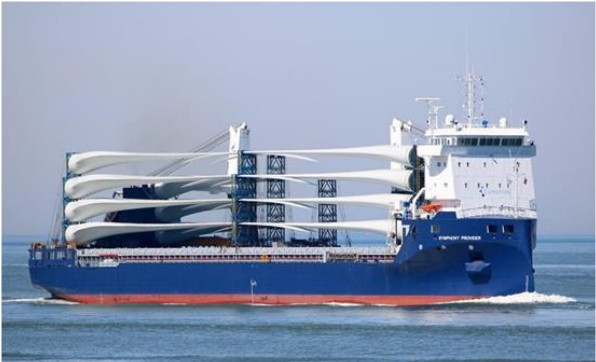
Figure 3.28: Blades transportation with a general cargo vessel (IMO: 9770713) [113]
