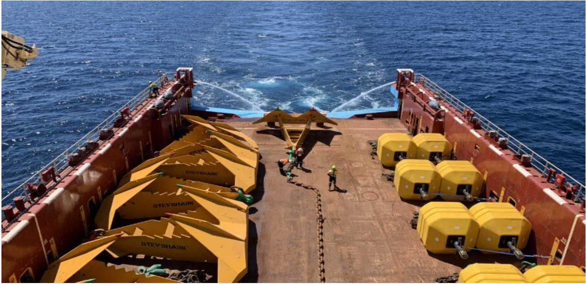
Figure 3.36: Anchors transportation in a vessel [119]
