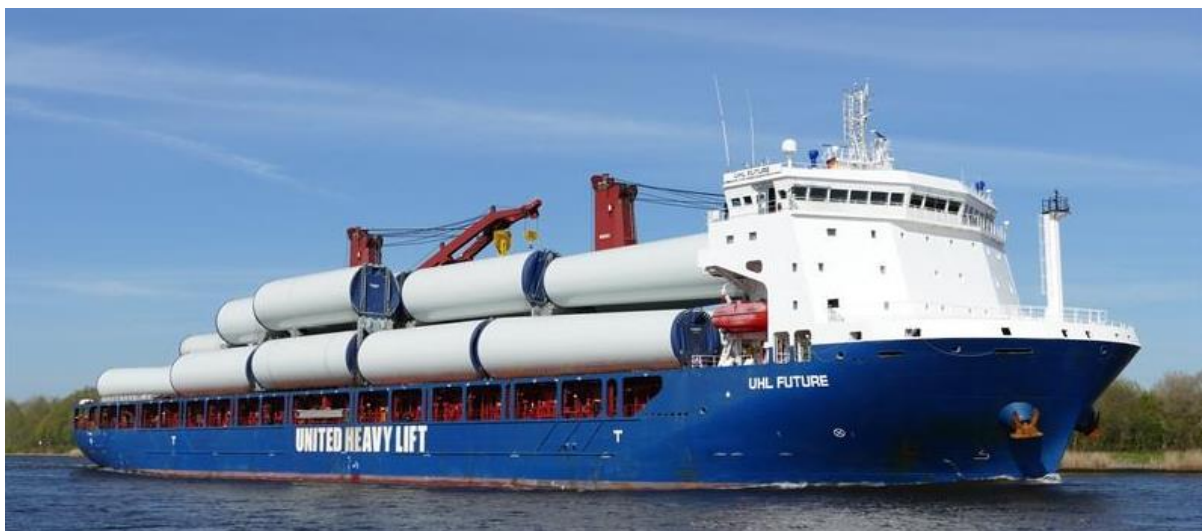
Figure 3.32: Tower offshore transportation [113]
