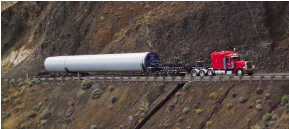
Figure 3.31: Onshore transportation of the tower [115]
