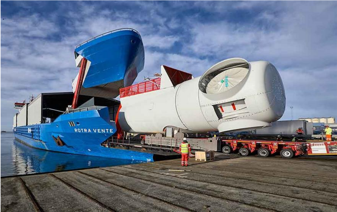
Figure 3.30: Loading of the nacelle to ROTRA VENDE for offshore transportation [114]
