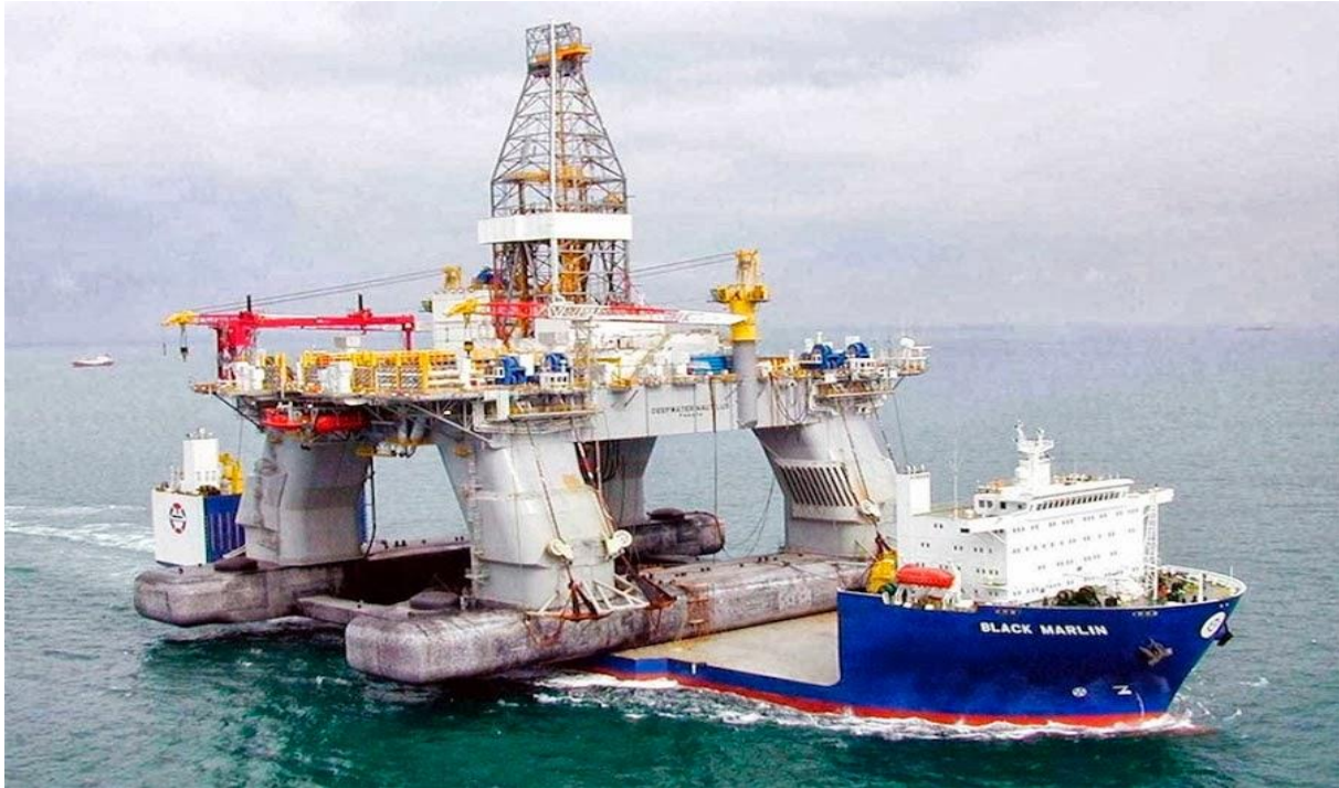
Figure 3.33: Offshore transportation with Black Marlin of a semi-submersible oil and gas platform [116]
