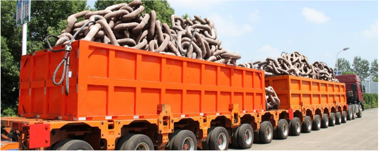
Figure 3.34: Onshore transportation of mooring lines [117]
