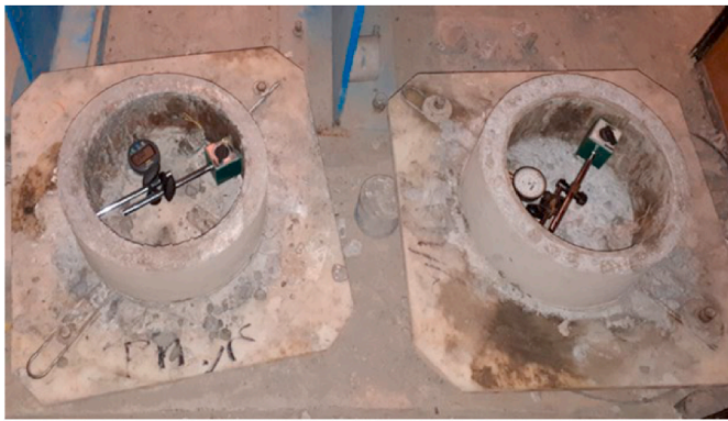
Fig. 11. Specimens ring test used in restrained drying shrinkage test.
