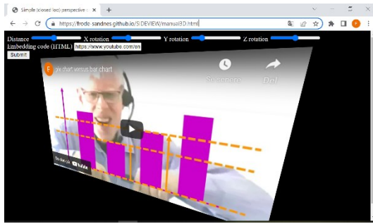
Figure 2: Manual calibration of approximate perspective correction of a YouTube video with 3D transformations.
