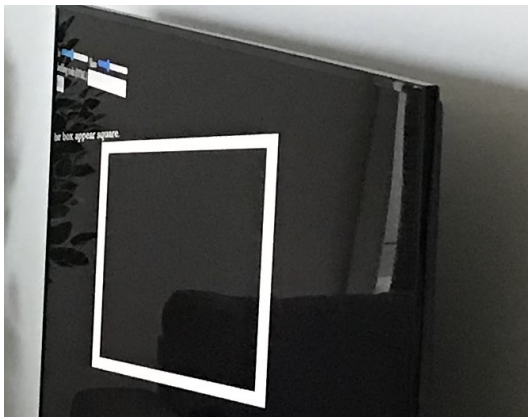
Figure 3: Partial perspective corrected calibration square from the viewers vantage point.
