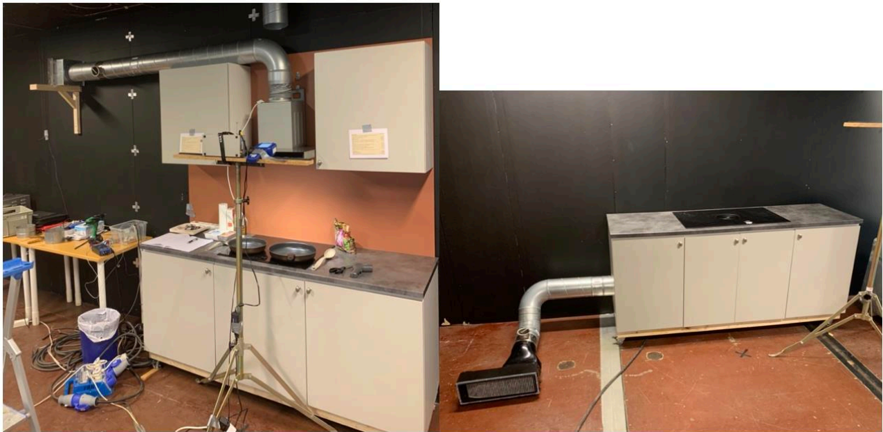
Figure 15 – Both Standard hood (left) and Downdraft system (right) in recirculation mode.
