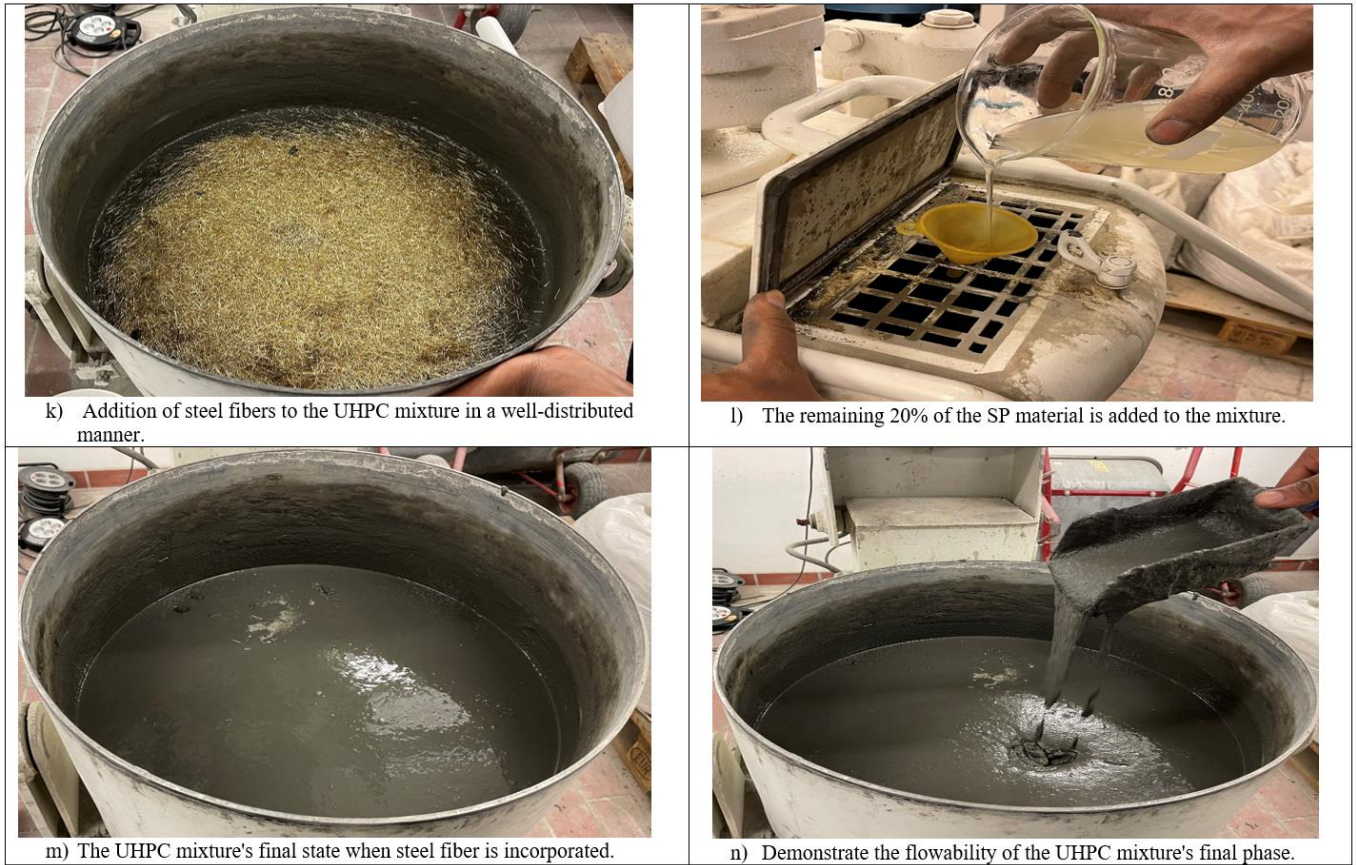
Figure 5.6 (k-n) Addition of steel fibers and the remaining superplasticizer
