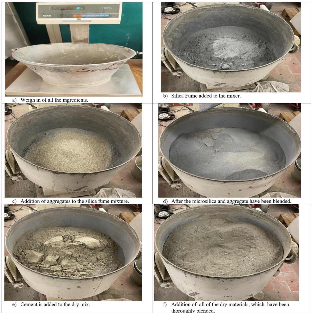
Figure 5.4 (a-f) Weigh-in and addition of the dry ingredients
