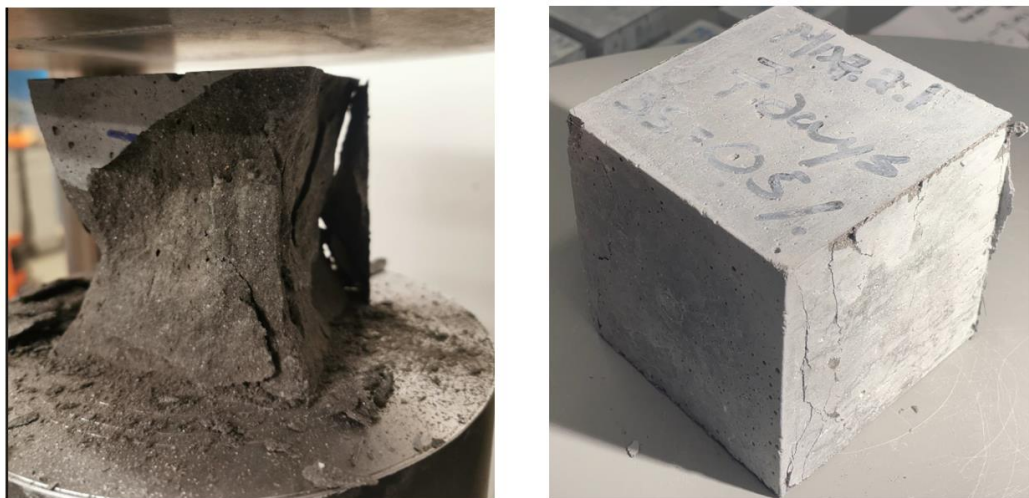
Figure 6.5 Failure appearance for UHPC specimen under uniaxial compression with (left) 0% steel fibre and (right) 0.5% steel fibre.
