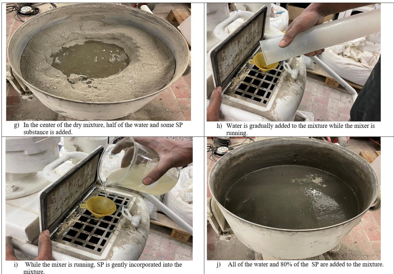
Figure 5.5 (g-j) Addition of water and superplasticizer
