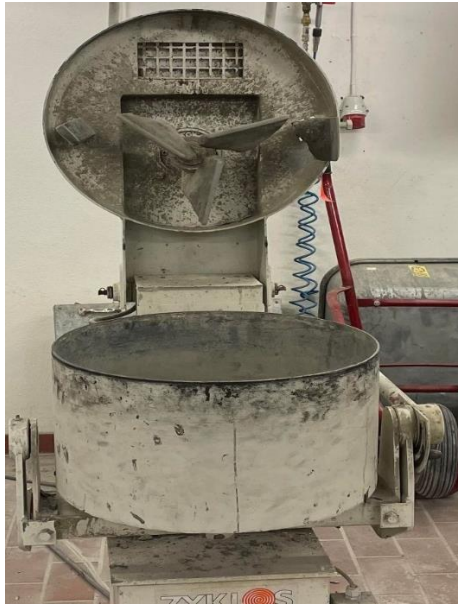
Figure 5.2 Zyklus ZK 30 E mixer used in this experiment
