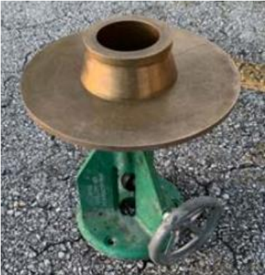
Figure 5.9 Flow table apparatus required in ASTM C1437 [33].
