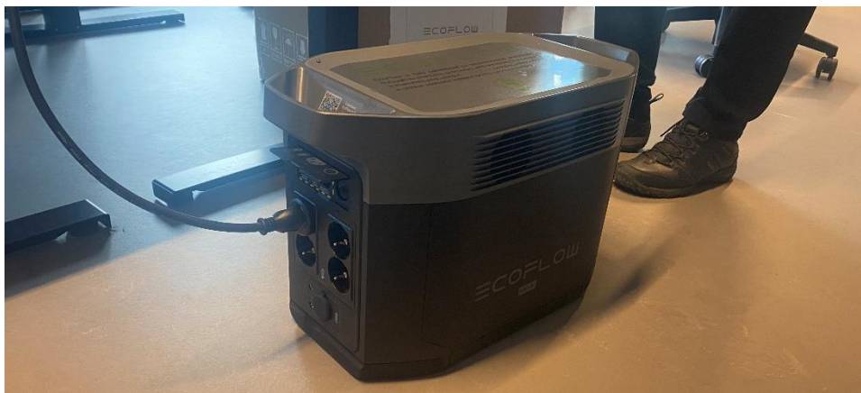
FIGURE 7: BATTERY USED FOR POWERING THE DATA GATHERING ON SITE
