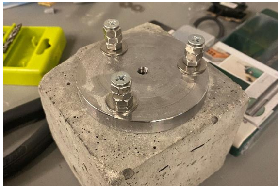
FIGURE 5: INSTALLED STEEL PLATE WITH THREE SCREWS ON A TRIAL CONCRETE CUBE
