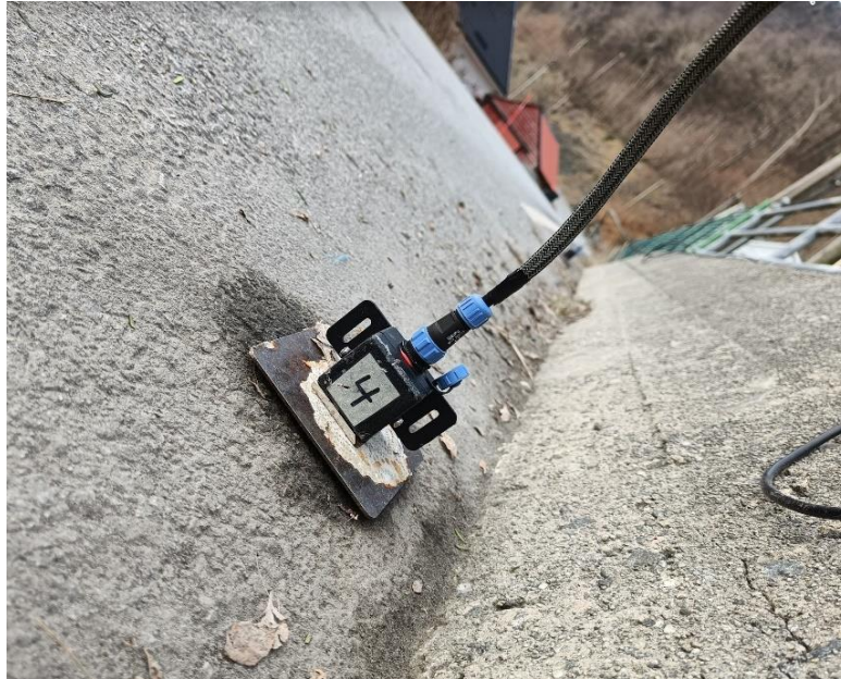
Figure 43 - Close-up illustration of one of the sensors attached to the steel plate
