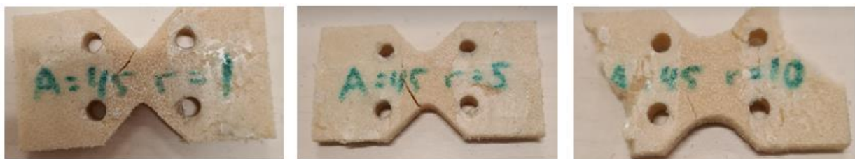
Figure 36: Samples with 45-degree angle and different radiuses. To the left radius 1. In the middle radius 5. To the right radius 10
