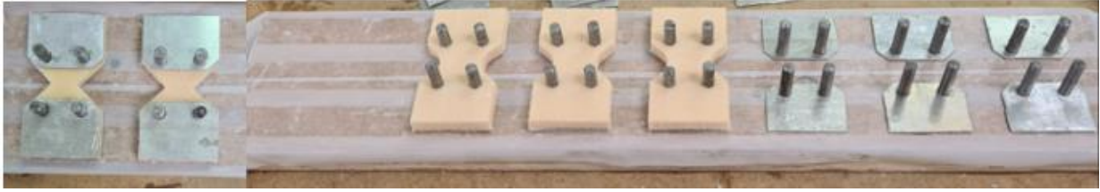
Figure 22: The gluing process. On the left, a shear sample with aluminium on the top and bottom. In the middle, samples with aluminium on the bottom. To the right aluminium plates with glue.
