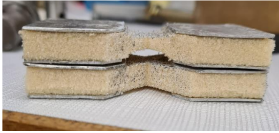
Figure 26: Bottom sample with 8mm thickness. Top sample with 4mm thickness
