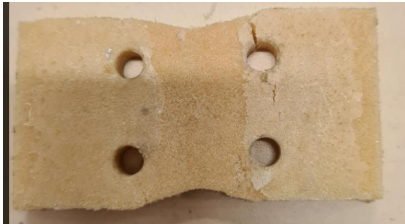
Figure 34: Sample representing the crack formation in 15- and 0-degree samples
