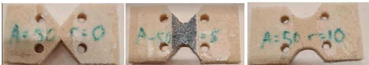
Figure 42: Samples with 50-degree angle and different radiuses. To the left: r=0. In the middle: r=5. To the right: r=10.
