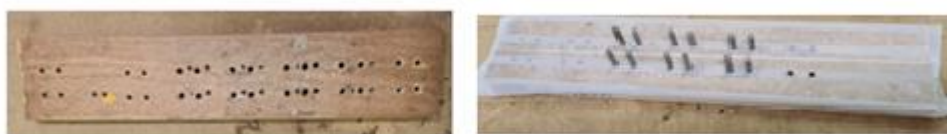
Figure 21: Wooden boards with holes made by CNC. One with metal cylinders (with plastic) and upper wooden plate (with soap)
