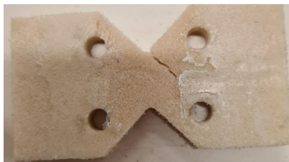
Figure 23: Crack development of sample with aluminium reinforced holes
