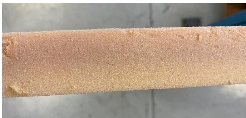
Figure 53: Divinycell H80 panel showing the variance in colour due to exposure to sunlight
