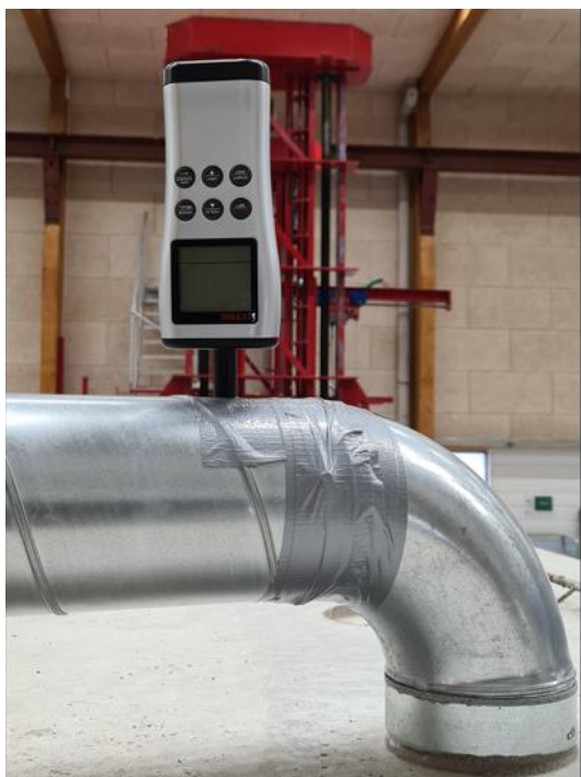
Figure 27: CP11 sensor measuring point no. 18.
