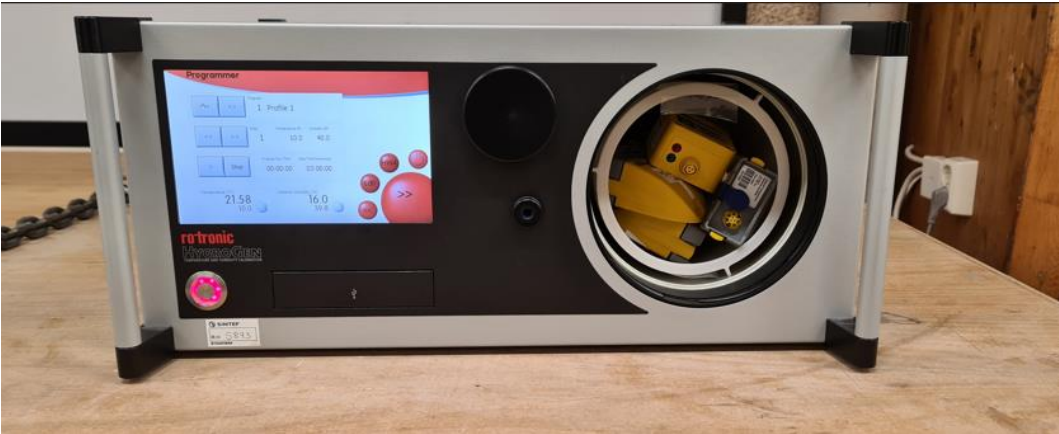
Figure 21: Rotronic device with the TinyTags placed inside relative humidity values.
