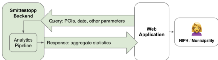
Fig. 3.3: High-level overview of the system’s aggregated statistics functionality, where coloured components indicate the scope of the backend solution.
