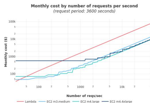
Figure 2.7 Cost Comparison in AWS on Lambda Vs. EC2 (BBVA, 2020)
