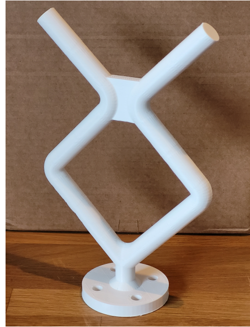
Figure 4.15: 3D printed fishtail handle drawn in Autodesk Fusion 360.
