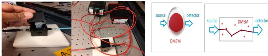
Figure 2. 3 Experimental arrangement for reflection-based measurement done In vitro liquid-based medium (a) Path of light in the medium (b) lab set up (c) Illustration of the light source and detector for transmission type of arrangement.
