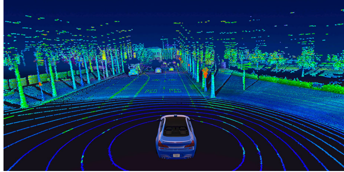
Figure 3.11: What a Lidar "sees" (Lidar, 2021).
