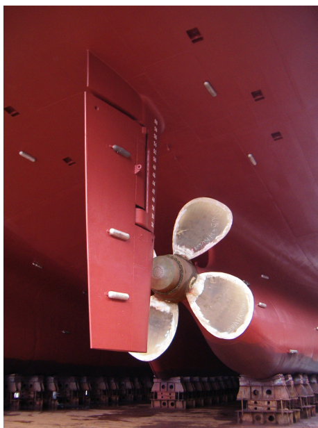
Figure 3.2: A propeller and a rudder (Wikipedia, n.d.-d)
