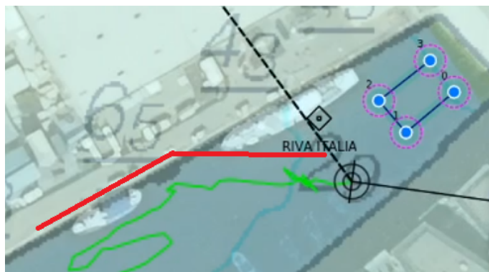
Figure 9.1: The path driven by the Otter is marked in green. A red supporting line is drawn to highlight the resemblance to the A* path found in figure 6.1. The Otter is symbolised as a bullseye
