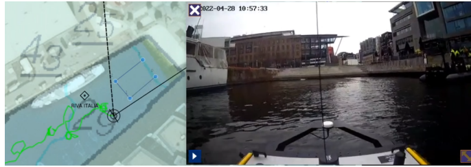
Figure 9.2: Left: The GPS position reported from the Otter. Right: An image frame taken from the Otter camera at the same time.
