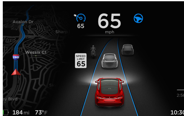
Figure 3.12: The Tesla autopilot (which is vision-based) in action, having detected two cars and a motorcycle (Falson, 2016)
