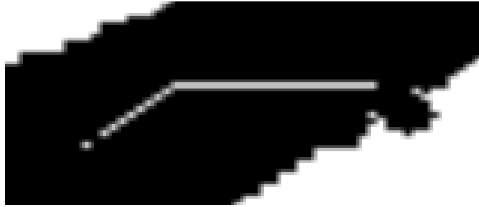
Figure 6.1: A binary representation of Filipstadkaia, where the A* algorithm has found a path to the entrance of the dock
