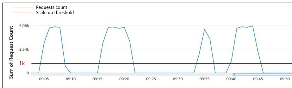
Figure 4.5: The sum number of requests received by each instance in a target group assigned to the Loadbalancer.
