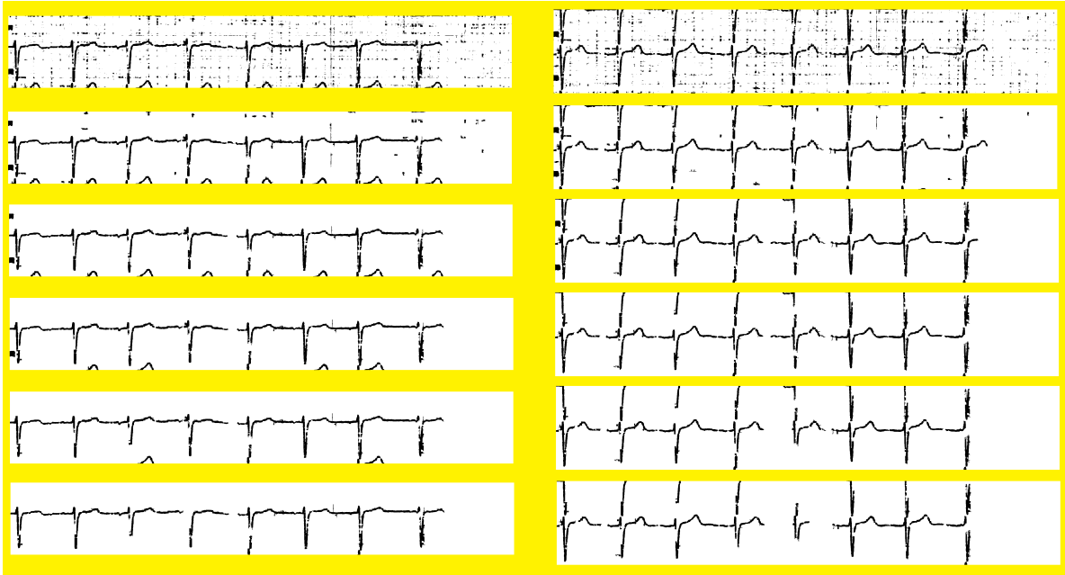
Figure 5.5: Effect of the different area size values of the CCL technique. For each screenshot these values increase from the top to the bottom. Left: first strip. Right: second strip.
