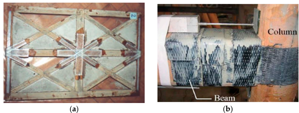
Figure 16. (a) Retrofitted timber frame walls with GFRP strips [115], and (b) a post and beam connection strengthened by CFRP strips [109].
