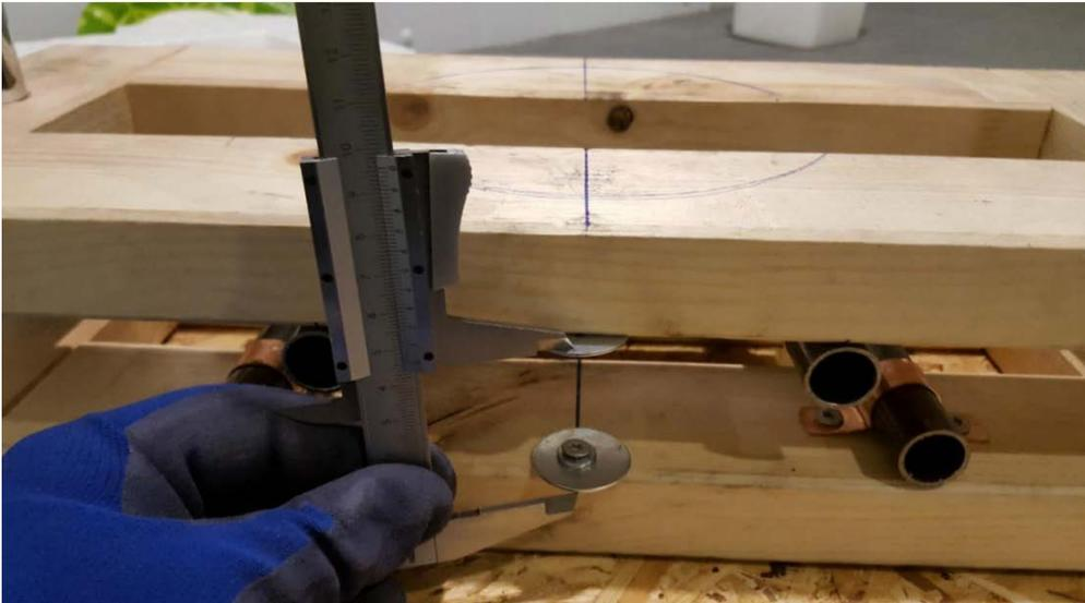
Figure 3: Recording displacement using a Vernier caliper. At this instant, the only load is from the upper frame alone. The middle of the frame is marked with a circle.
