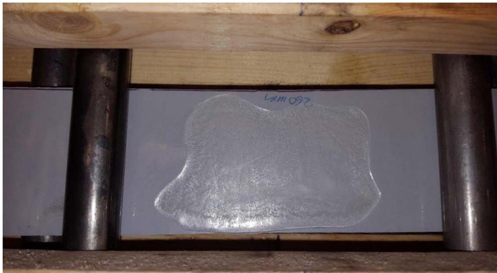
Figure 2: ice on polyurethane
