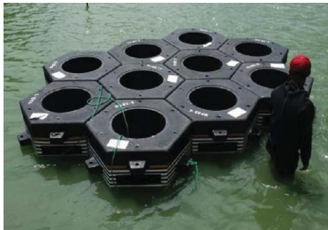
(a) Modular units for floating wetlands
