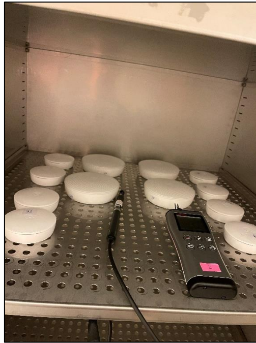
Figure 7. An ongoing calibration procedure of the Airthings sensors
