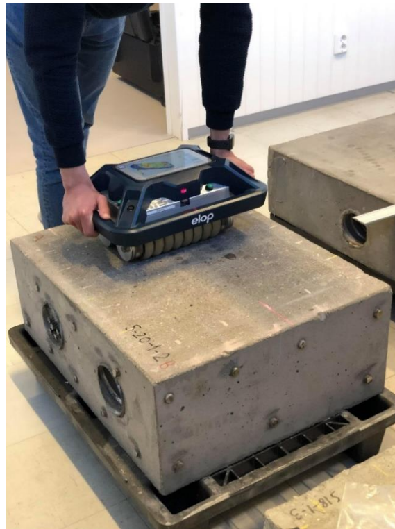
Figure 75 Scanning S-20-1-2 B with laser pointing on the center chalk marking
