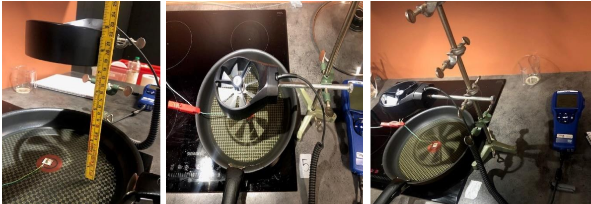
Figure 22: Measurement setup for air velocity and temperature in the plume
