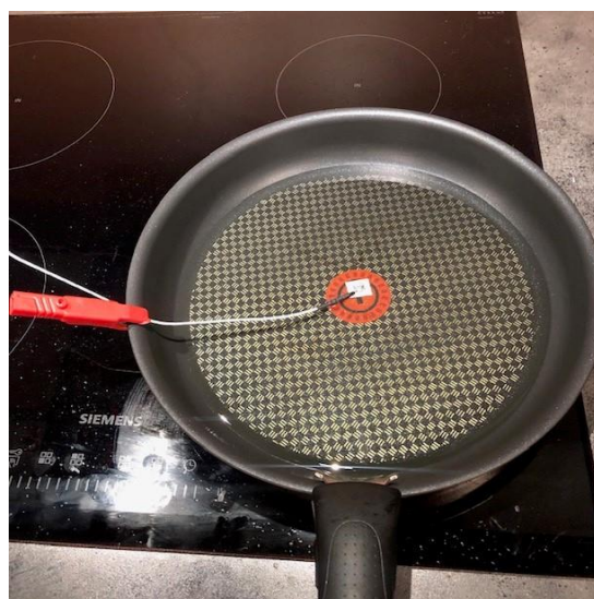
Figure 20: Test equipment; pan with the heated oil
