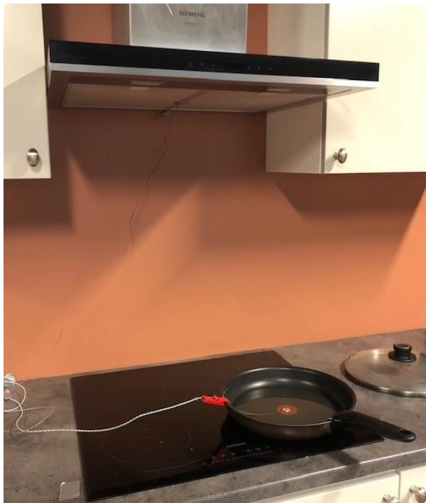
Figure 9: Experiment setup: range hood, cooktop, and equipment
