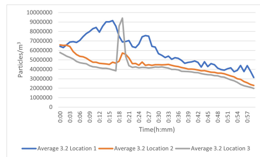
(d) Raw Aerotrak measurements, averaged values from all three tests 3.2
