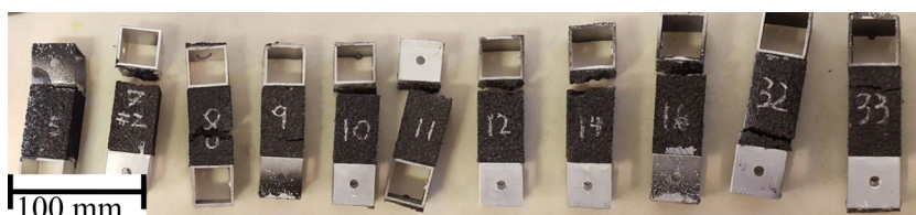
Fig. 9. Samples tested in tension at different temperatures. Sample 8 illustrates failure within the material, while sample 10 is an example of bonding failure.
