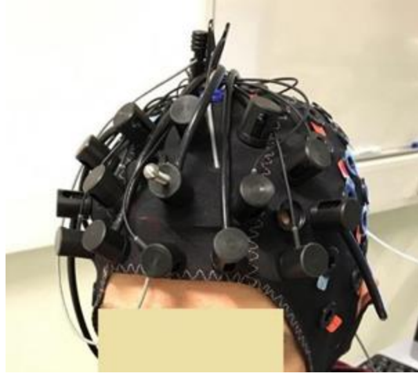
Figure 3-11 Detector 4 with the Spring-loaded grommet and a screw
