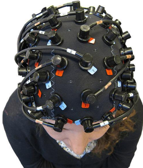
Figure 3-5 fNIRS cap with the implemented optodes (NIRS Caps & Probes, n.d.)
