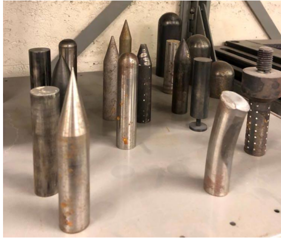
Figure 9: Different kind of projectiles used in experiments at NTNU [photo taken by author].
