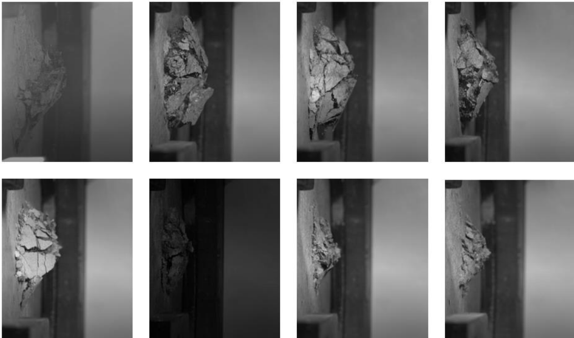
Figure 26: Projectile exiting C35 concrete plate for initial velocity from top left corner: 119.7 m/s, 137.7 m/s, 143.0 m/s, 155.3 m/s, 185.0 m/s, 206.4 m/s, 245.0 m/s, 294.3 m/s.
