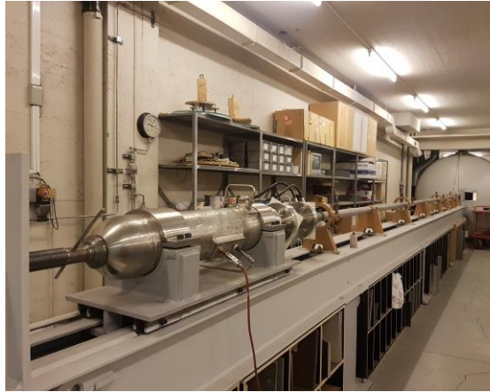
Figure 18: Overview of the pressure tank, barrel and the closed impact chamber.
