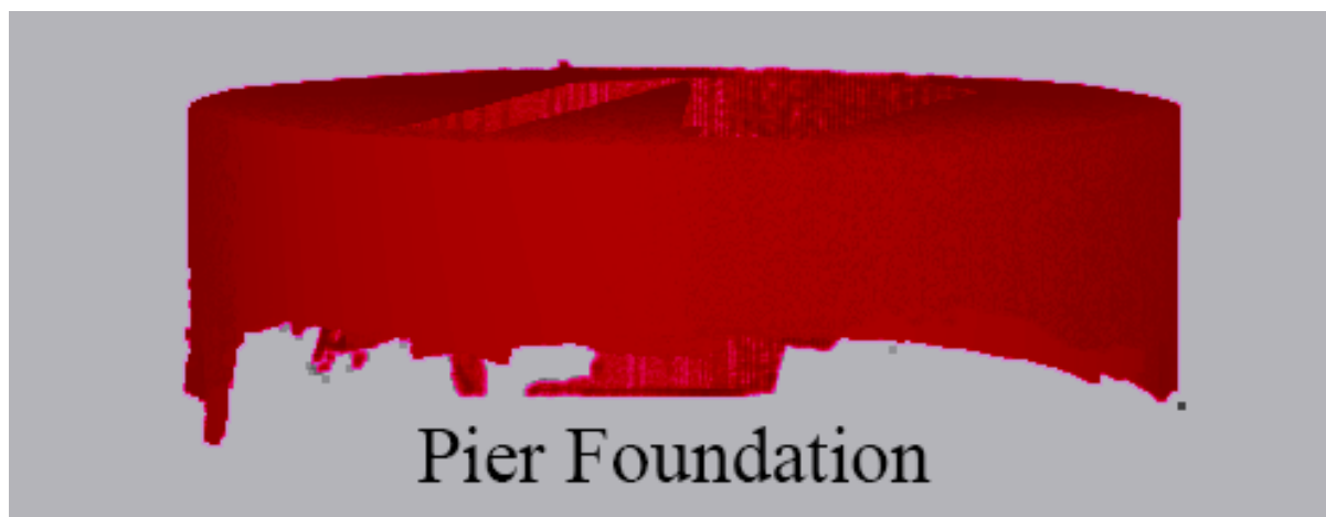
Figure 4.17: The point cloud of the pier foundation
