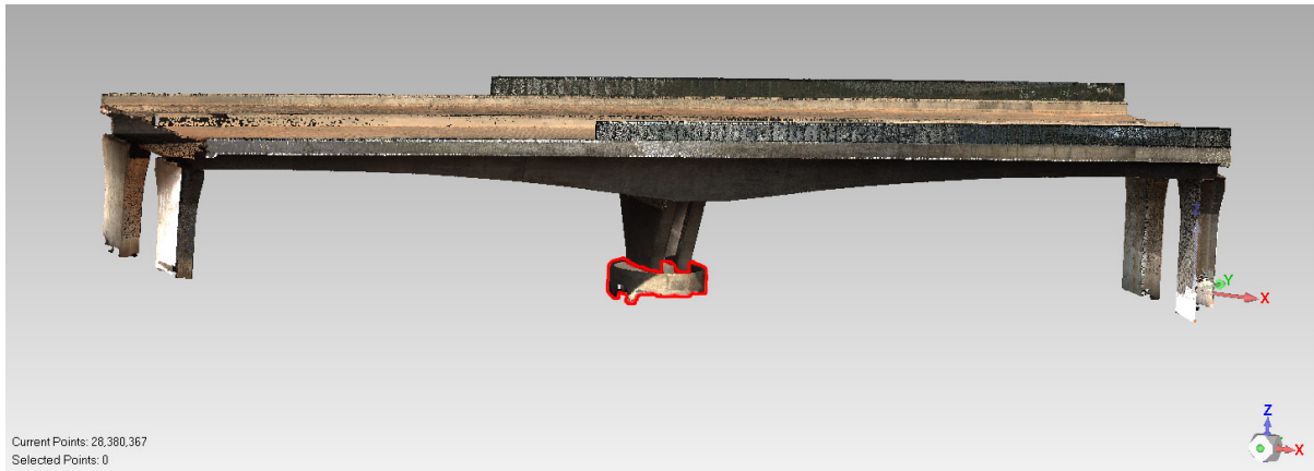
Figure 5.26: The point cloud of the Dade Bridge with its pier foundation outlined in red
