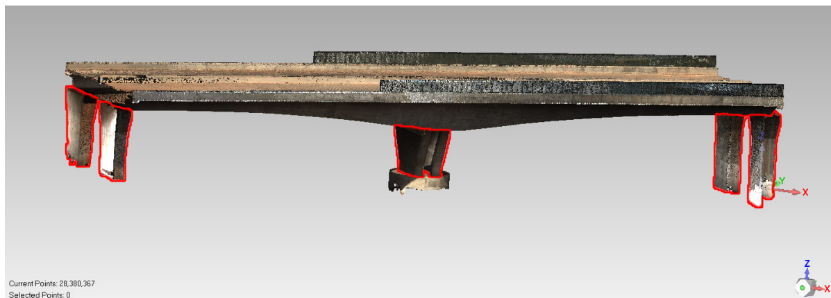
Figure 5.18: The point cloud of the Dade Bridge with its pier columns outlined in red
