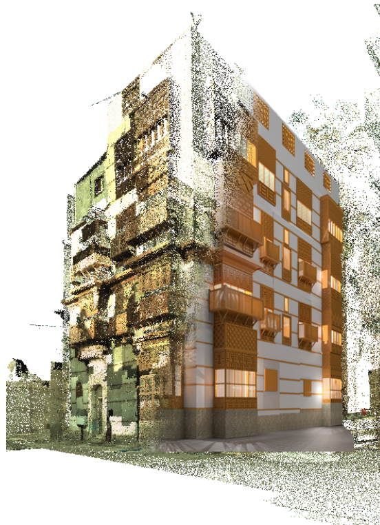
Figure 1.2: Reverse model based on point cloud data [1]
