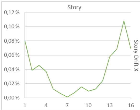
Figure 5-59 Story drift from direct integration T-H for Dursun X of MBF
