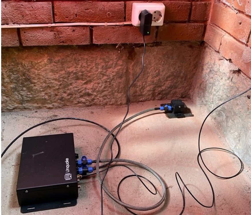
Figure 44 Sensor and datalogger - initial testing
