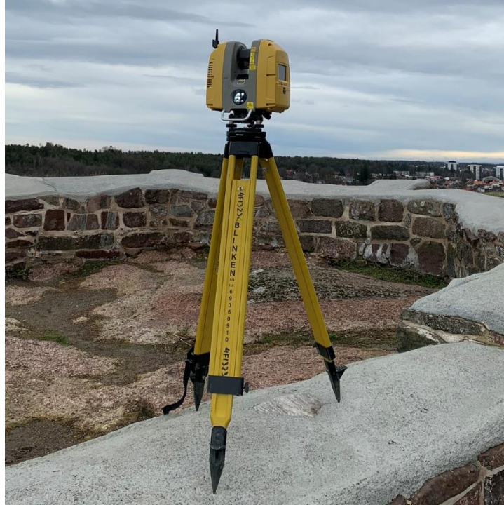
Figure D. 7 3D laser scanning 01
