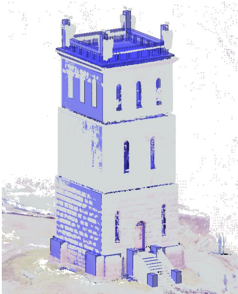
Figure 21 Recap point clouds in Revit
