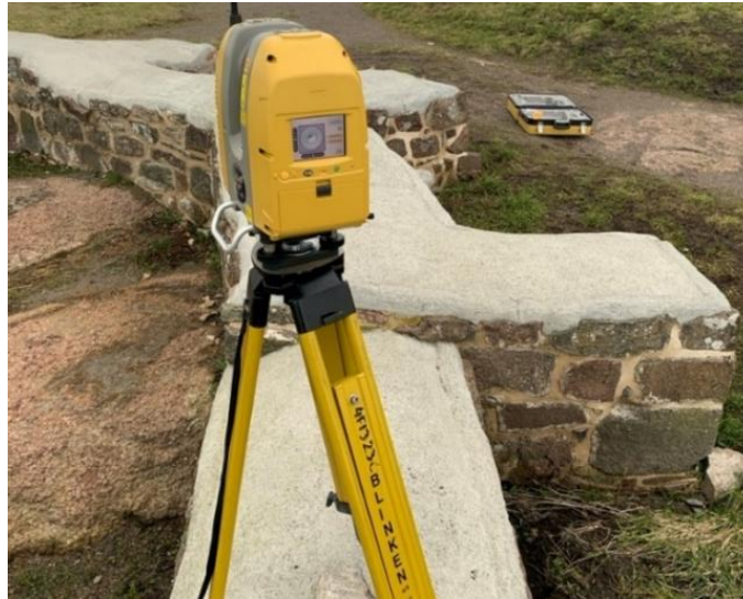
Figure 19 3D laser scanner calibration
