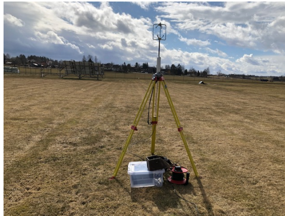
Figure 3.4: Ultrasonic anemometer under operation.
