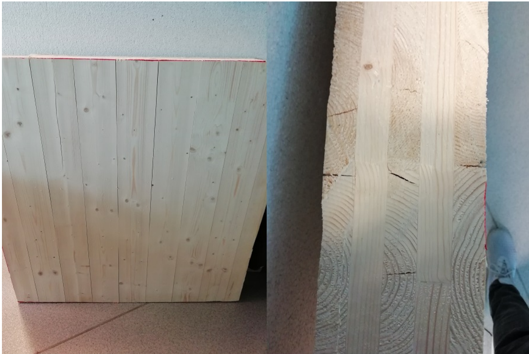
Figure 21: Cross-laminated timber element from Splitkon
