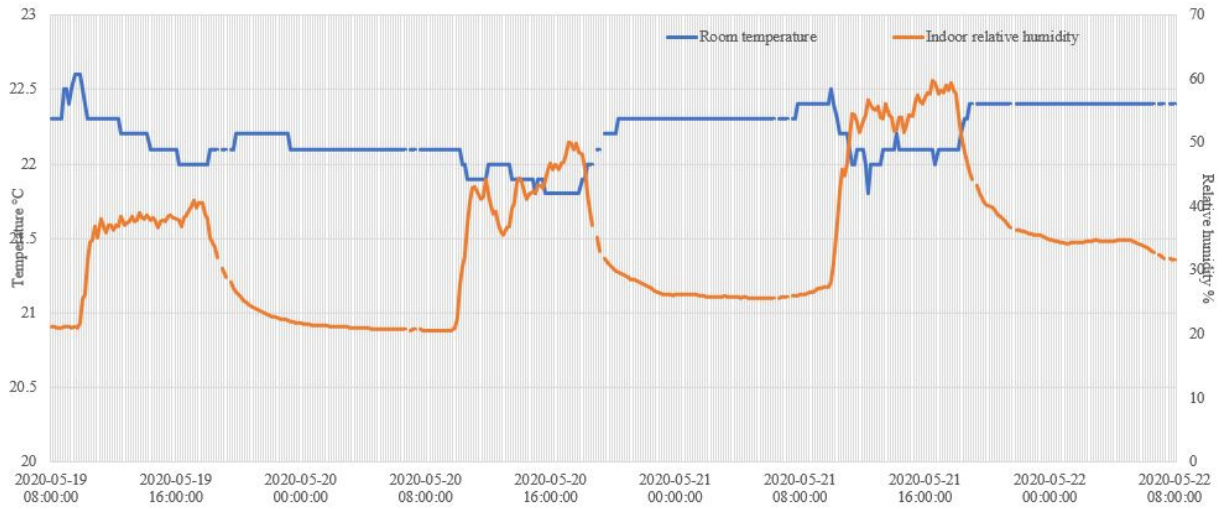
Figure 53: Room temperature and relative humidity relationship Splitkon (Celsicom)
