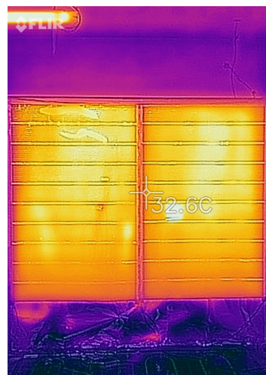
(b) Thermal image of the heating foil activated.
