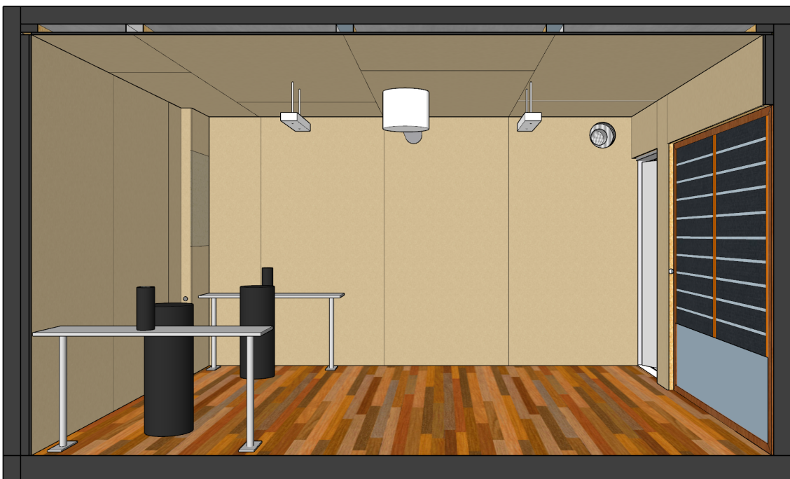
Figure 2.6: The climate room with the heat gains.
