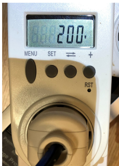
(a) Heat foil sizing verified with an electrical power meter.
