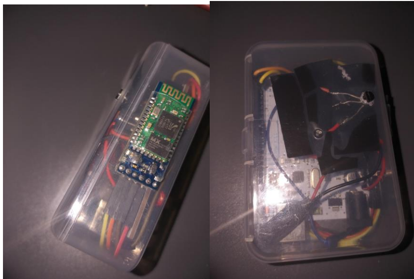
Figure 4: Image of Arduino connected with Bluetooth
