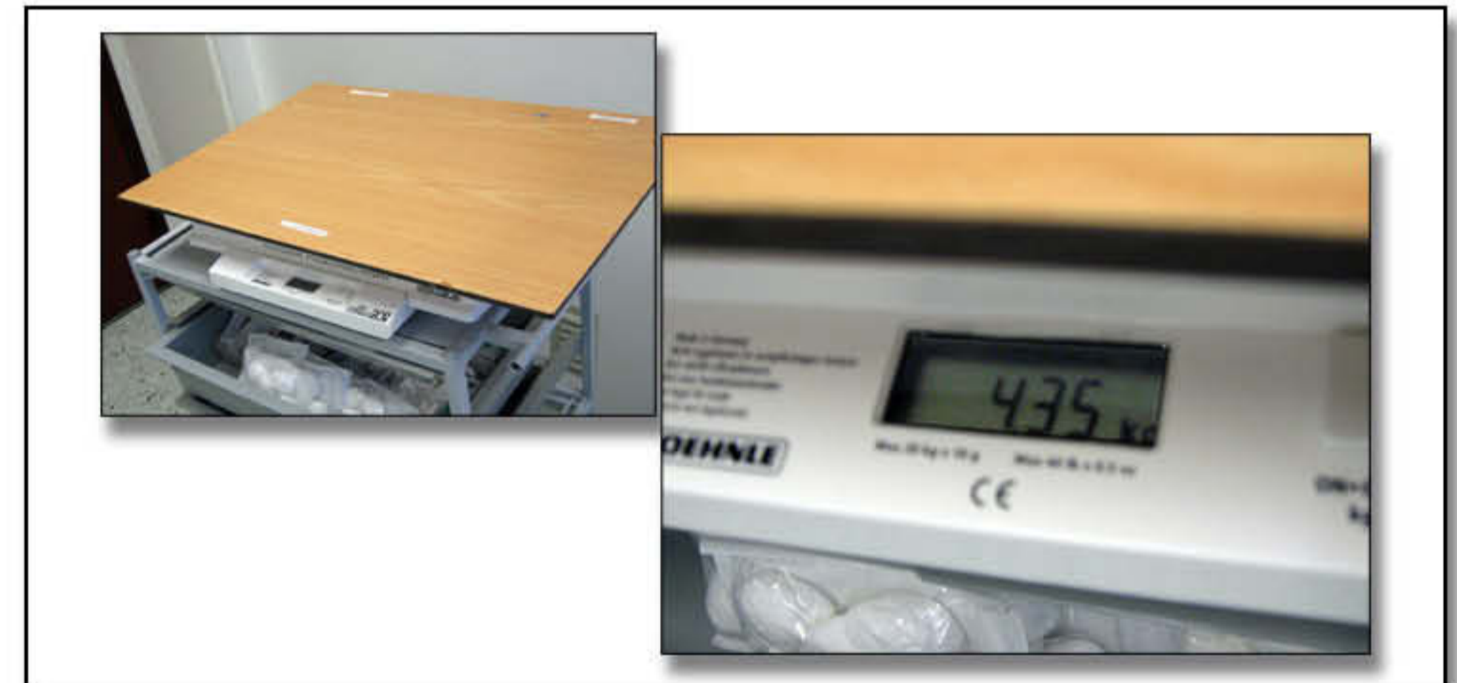
Figure 12: the weight of existing CPR board
