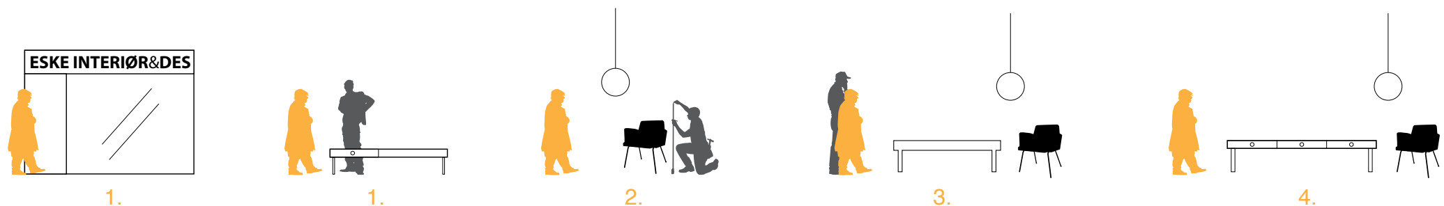
ill. 5.2 / 'bespoke furniture' initial project based on a non-grid, seamless system, measured to fit the customer by the millimeter. 1/ the customer is presented with the system 2/ house call by carpenter or trained salesperson looking into use and context - measuring 3/ rough scale model based on customer specifications and measures - final adjustments 5/ furniture delivered.
