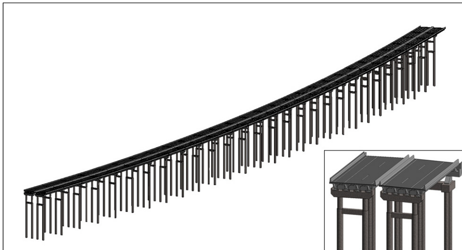
Figure.5 Bridge quality control BIM model
