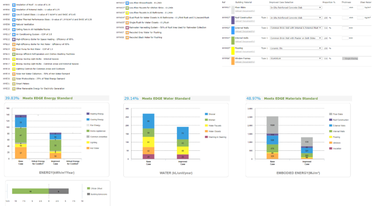
Figure 11. Three screenshots of inputs and outputs for energy use (left), water use (middle), and embodied energy (right) in the EDGE tool [30]
