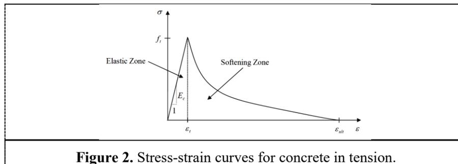
**Figure 2.** Stress-strain curves for concrete in tension.
