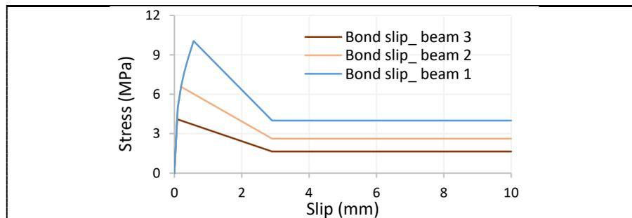
**Figure 3.** Bond slip behaviour of the reference beam (no.1) and the corroded beams (no.2 and 3).
