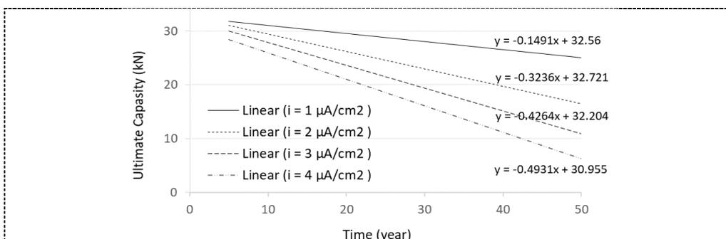
**Figure 5.** Trendlines of ultimate capacity vs time for the corroded RC beam with different current rates of corrosion: a)  $i = 1 \mu\text{A}/\text{cm}^2$ , b)  $i = 2 \mu\text{A}/\text{cm}^2$ , c)  $i = 3 \mu\text{A}/\text{cm}^2$  and d)  $i = 4 \mu\text{A}/\text{cm}^2$ .
