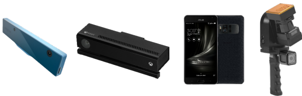
Fig. 5 From the left: Intel RealSense ZR300, Microsoft Kinect v2, Asus ZenFone AR, ZEB-REVO. Not in correct sizes.
