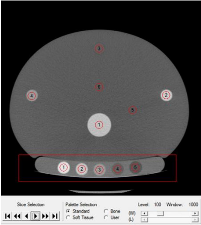
Fig. 1. Illustration of volume of interest placement in the quality assurance phantom, Mindways Solid.
