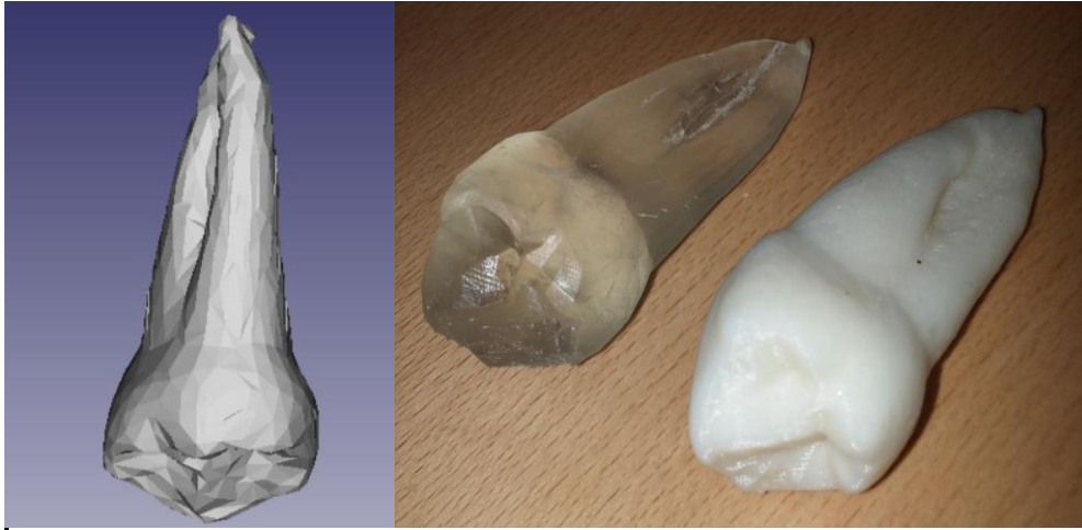
Figure 4. Showing an example of a micro CT (computer tomography) image of human tooth with its printed results from Formlabs printer ( transparent) and Maker Boot ( white). The length of the tooth is about 20mm.
