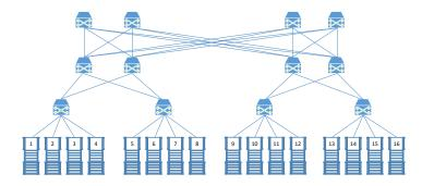
Figure 7: The VL2 data center network model used in the simulations.
