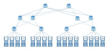
Figure 5: The Tree data center network model used in the simulations.
