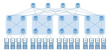
Figure 6: The Fat-tree data center network model used in the simulations.
