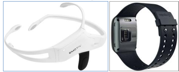
Figure 3: Emotiv Insight (EEG headset) and wristband Empatica E4 (electrodermal and cardiovascular activity)
