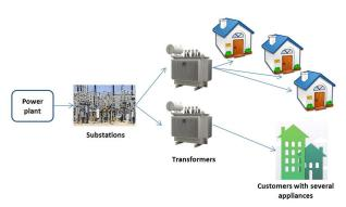
Fig. 2: A high level structure of the power grid.
