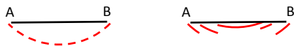
Figure 4. Reducing the height of the arc by splitting the arcs in sections.
