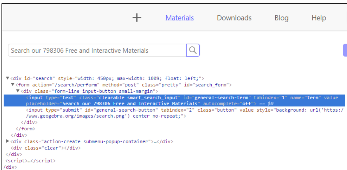
Figure 4-5: Search Field and Search Button do not have name and value respectively describing its purpose
