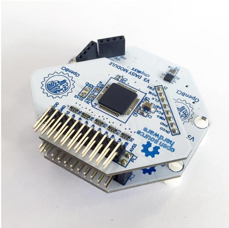
Figure 9 OpenBCI. (Photographer). (2017, May 14). Picture of the Cyton + Daisy Biosensing Boards (16-Channels) [digital image]. Retrieved from <https://shop.openbci.com/collections/frontpage/products/cyton-daisy-biosensing-boards-16-channel?variant=38959256526>
