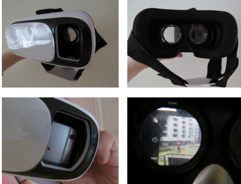
Fig. 2. Variation on Google cardboard for AR using the mobile camera.
