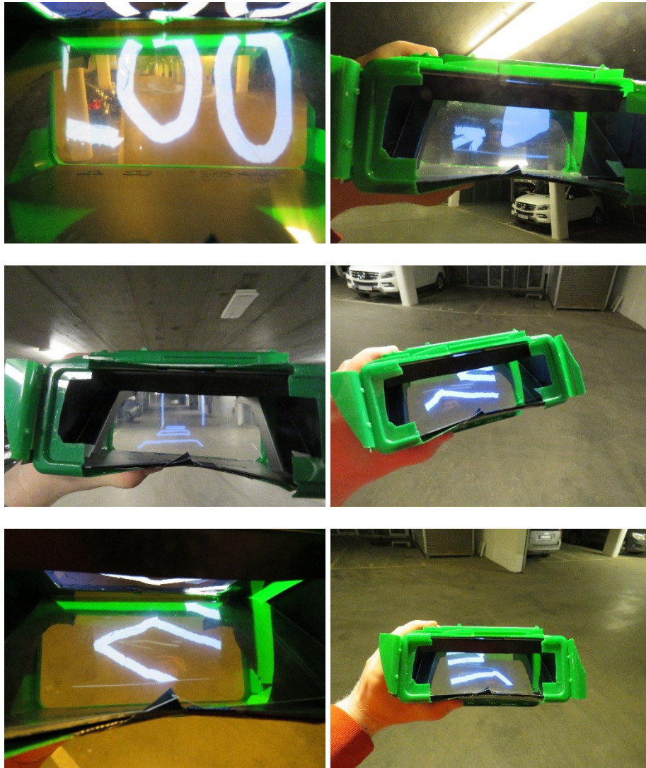
Fig. 12. Panoramic sketches superimposed on the real-world views. The four examples in the middle row and bottom row show the outline of a zebra crossing and a virtual gate.
