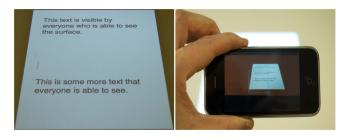
Figure 3. The image on the left shows the surface as everyone sees it. The image on the right is seen through the device (in this case an iPhone), revealing more information than could be seen just by looking at the surface.
