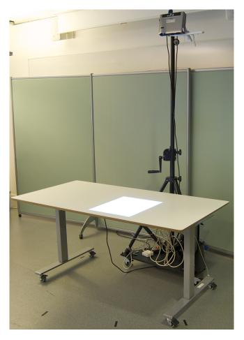
Figure 1. This image shows the system setup. It consists of a projector mounted on a stand, projecting the image on to the top of a white table. It is possible to interact with the table in a variety of way, including mouse, keyboard and hand held devices (e.g. iPhone). It is both possible and desirable to add touch functionality, but our prototype does not support this as of the time of writing.
